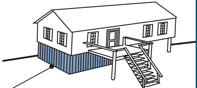
4. ELEVATED BUILDING WITH ENCLOSURE
